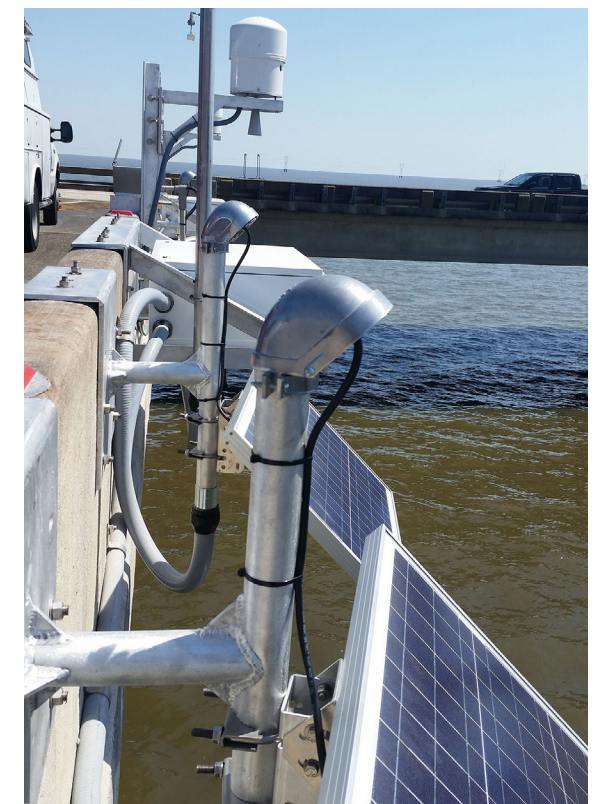
This PORTS ® station will provide real-time, 24-hour water level information to mariners, providing safe transport in and out of Port Fourchon, Louisiana.
