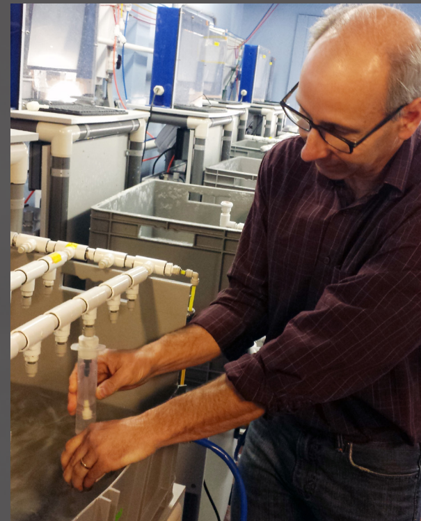
In the ocean acidification laboratory at the NOAA Mukilteo Research Station, Dr. Paul McElhany demonstrates the functionality of the equipment that exposes California Current species to ocean acidification, temperature change, and deoxygenation treatments.
